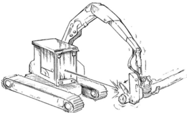
**Figure 2.** Chain shot: A link of chain snapping and being flung off the cutter bar (in this case, towards the machine operator) (WorksafeBC, 2004).
