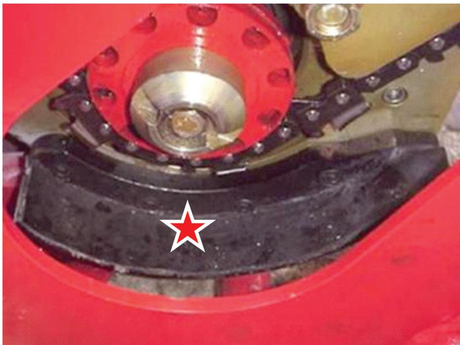
**Figure 1.** Chain shot guard (shown by the star on the picture) (adapted from New Zealand Department of Labour, 2005)
