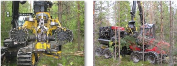
Fig. 5. The cutting of whole-trees and delimbed longwood was carried out using a conventional harvester head equipped with multi-tree-handling accessories (left). Bundle harvesting was carried out using the newly-developed Fixteri bundle harvester (right).
