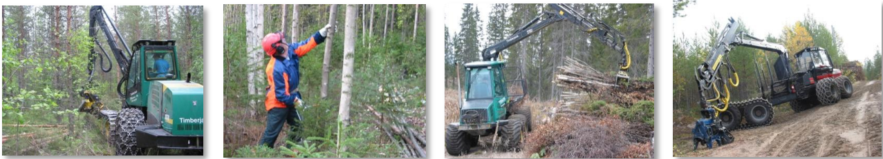
Fig. 1. Mechanised cutting with a harvester (left) or manual cutting by a logger (2 nd on the left) is combined with mechanised forwarding (2 nd on the right), whereas a harwarder (right) performs both harvesting and forwarding simultaneously.
