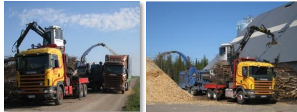
Fig. 6. The harvested wood was chipped either at a roadside landing (left) or at a terminal using a trailer-mounted drum chipper (right).
